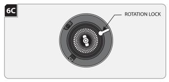
**NOTE:** Lamp housing can rotate 361° horizontally.
