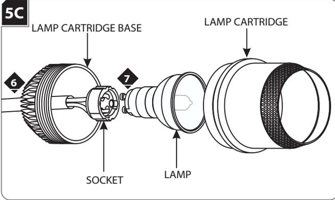
Use **ONLY** 120 Volt, 20 Watt GX10 Base MR16 Ceramic Metal Halide lamp.
