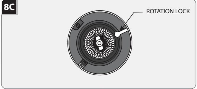
**NOTE:** Lamp housing can rotate 361° horizontally.
