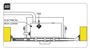
Replace the electrical box cover. Make sure that the top edge of the cover snaps under the tab.
