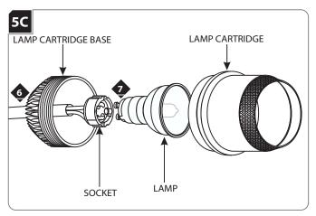
Use **ONLY** 120 Volt, **20** Watt GX10 Base MR16 Ceramic Metal Halide lamp.
