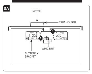
Slightly loosen the wing nut to slide the butterfly bracket up or down.
