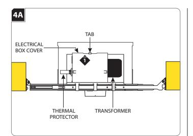
Push the tab on the housing electrical box up and remove the electrical box cover.
