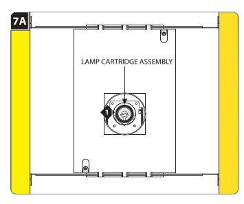
1 Pull the snoot to remove the lamp cartridge assembly.
