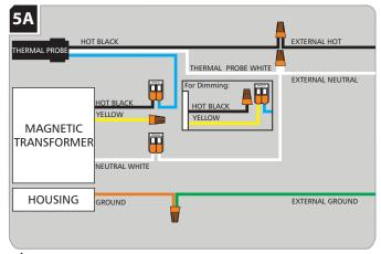
Connect the neutral power line wire to the white transformer wire and the white thermal probe with a wire nut.
