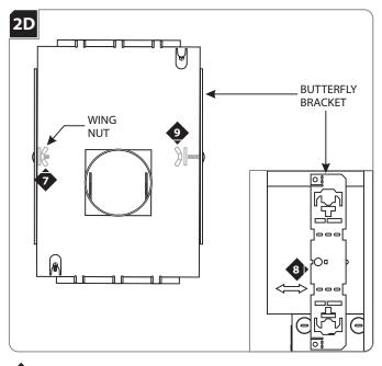
6 Attach the wing nut loosely to the button head screw.
