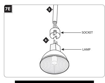
Use MAX 75 Watt Type MR16 Halogen Lamp.
