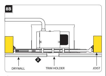
2 Align the cut out section of drywall with the trim holder and install drywall.
