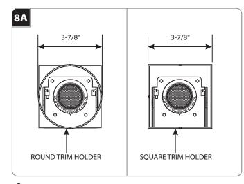
**1** For round trims, mark a 3-7/8" diameter circle on drywall. Cut out the marked section.
