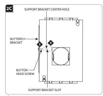
Place the support bracket center hole onto the button head screw.
