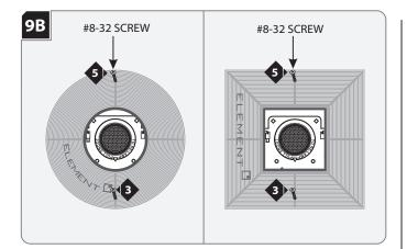
3 Secure the plaster ring in place with the two provided flat head #8-32 screws. Make sure that the screws penetrate through the drywall into the housing screw holes.
