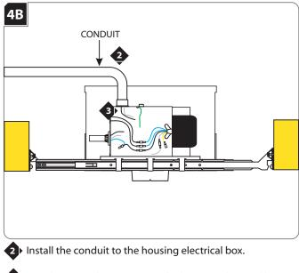
3 Run the power line wires into the housing electrical box.
