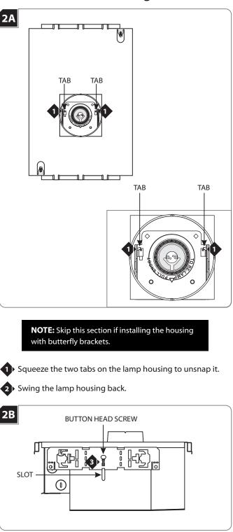
Place the button head screw through the square cut out of the butterfly bracket into the housing slot.
