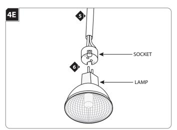
Use **MAX 75** Watt Type MR16 Halogen Lamp.
