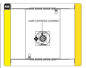
Pull the snoot to remove the lamp cartridge assembly.
