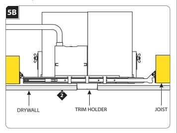
Align the cut out section of drywall with the trim holder and install the drywall.
