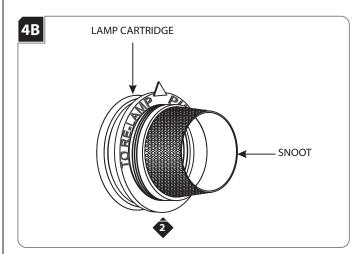
Unscrew the snoot from the lamp cartridge.
