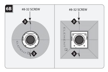
Secure the plaster ring in place with the two provided flat head #8-32 screws. Make sure that the screws penetrate through the drywall into the housing screw holes.
