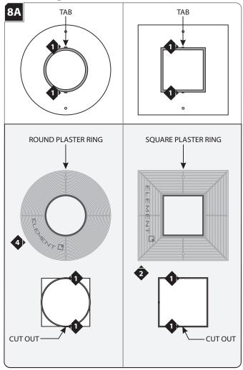
1 Line up the two tabs in back of the plaster ring with the two cut out sections of the trim holder inside edge.
