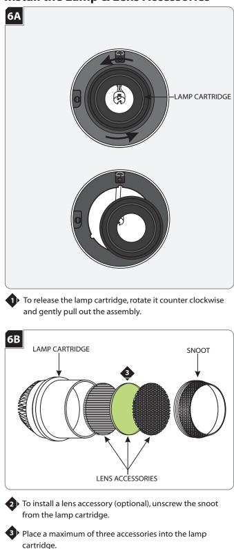
• Replace and tighten the snoot completely to the lamp cartridge.
