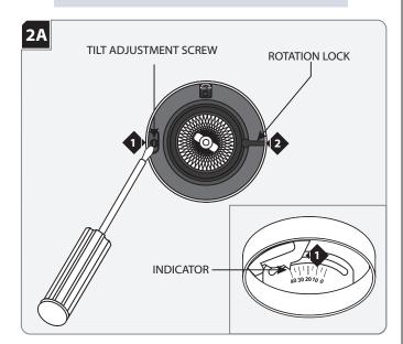
1 The lamp housing must be adjusted out of the way in order to install the butterfly brackets: tilt the lamp housing to the maximum angle by rotating the tilt adjustment screw.
