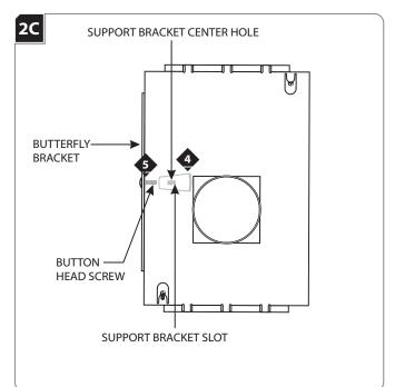
Place the support bracket center hole onto the button head screw.
