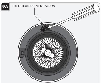
To adjust the height rotate the height adjustment screw. Adjust upward to minimize glare and flash on the trim or downward for maximum light output and efficiency.
