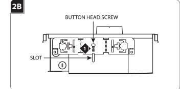
3 Place the button head screw through the square cut out of the butterfly bracket into the housing slot.
