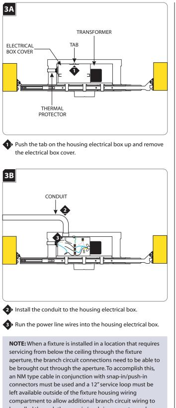
be pulled through the snap-in/push-in connector and extended out through the aperture below ceiling level.
