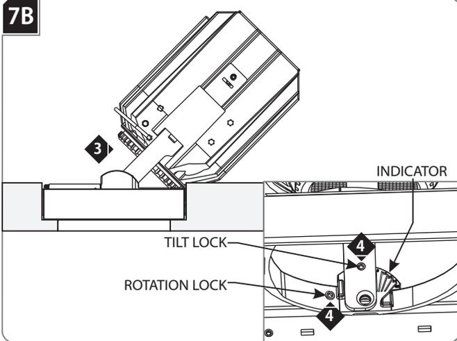
**NOTE:** Module can rotate 361° and tilt to 45°. For proper wall wash positioning, tilt until 15° angle is reached.
