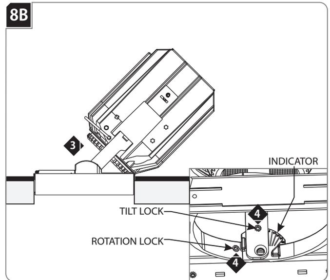
**NOTE:** Module can rotate 361° and tilt to 45°
