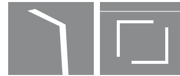
Wall-to-Ceiling Transition (Recessed only)
