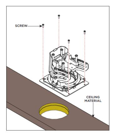
3. Attach the mechanism to the ceiling material with the four (4) Philips screws provided.
