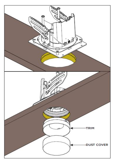
Use the dust cover as a guide to locate the mechanism in the center of the opening. If a trim is available, remove the dust cover and test fit it to ensure the mechanism is centered over the opening. Be sure to replace the dust covers once the fixture is installed.
