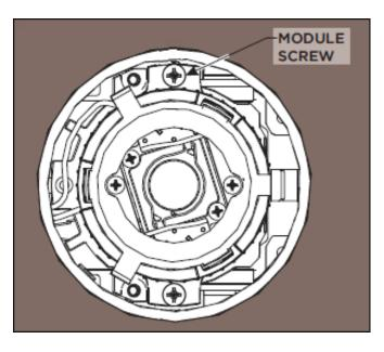
6. Mount the light module assembly to the mechanism using the two (2) module screws.
