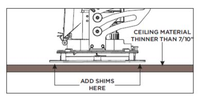
If the ceiling material is thinner than 7/10", place shims under the 4 holes in the mounting plate to raise it up to approximately 3/4" above the roomfacing (bottom) surface.
