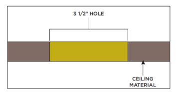
4. Cut the opening in the plank following best routing practices. The hole in the plank will be approximately 3.5" across.
