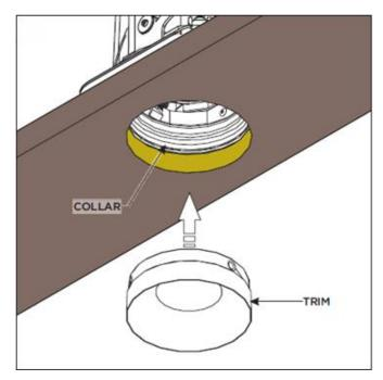
1. Push the trim up into the opening in the ceiling until it snaps into the sliding collar inside the mechanism.
