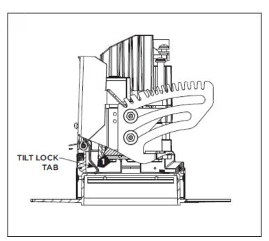
1. To unlock the tilt, pull tilt lock tab towards optic.
