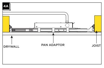
Install the drywall keeping note of the location of the housing's opening
