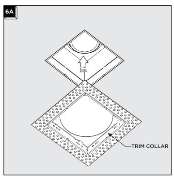
Push the trim collar into the ceiling cut-out until the bottom of the collar is flush with or slightly above the bottom of the ceiling.
