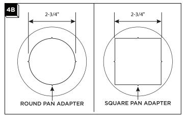
**2** For round trims, mark the location of the 2-3/4" diameter circle on drywall. Use the inside edge of the housing pan adapter as a guide to cut the hole.
