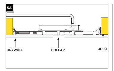
Note: The fixture will accommodate a 1/2" to 1-1/4" ceiling thickness.
