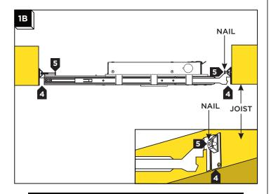
**NOTE:** The adjustable bars can be mounted to joists that are spaced 16" - 24" apart.
